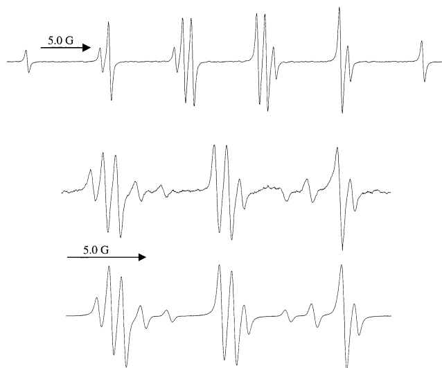
FIGURE 1. Experimental EPR spectrum of nitroxide 6b in benzene at room temperature (above). Below it is shown a portion of the experimental EPR spectrum obtained by partial oxidation of a mixture of 6a and BHT and its computer simulation.
